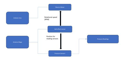
Figure 11: A schematic picture over the structure for the code controlling the system. This is implemented using Arduino IDE and the complete code can be found in Appendix A.
