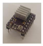
Figure 10: The stepper motor driver DRV8255.
