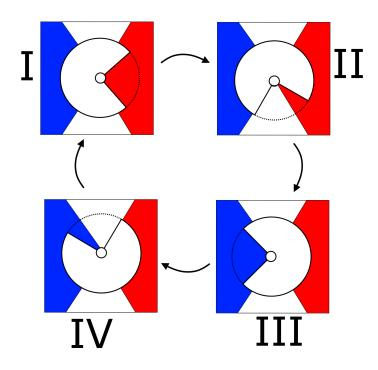
Figure 2: Illustration of a cycle of the GREC. Red part illustrates the heat source, and the blue part the cold source.
