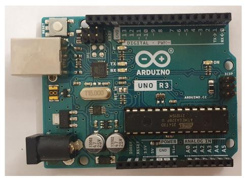
Figure 5: A picture taken with cellphone camera showing the Arduino Uno used for the project.
