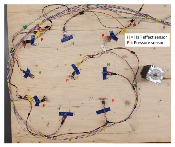
Figure 13: A test assembly of the approximate placement of the sensors in the GREC. A drawn RS is shown on a wooden plate to illustrate where the sensors are placed.
