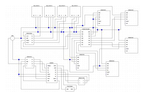
Figure 12: Figure showing the wiring diagram designed of the components for the GREC. For a clearer picture, see Appendix B
