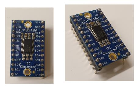
Figure 7: The I2C Multiplexer component.
