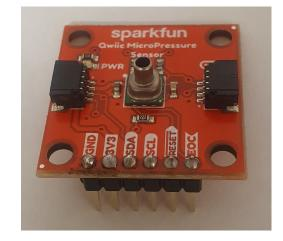
Figure 6: The micropressure sparkfun sensor.
