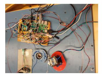
Figure 3: A picture of the current electric system for the GREC. A stepper-motor glued to a red plate is visible in the picture as well as the Arduinos and the Raspberry Pi
