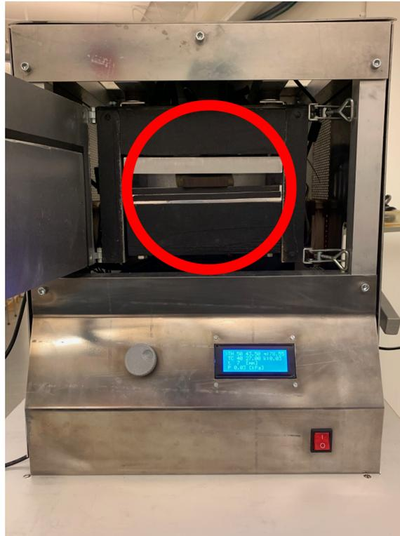
Figure 7: HTC-testing setup, the red circle highlights the material specimen and its placement for the test.
