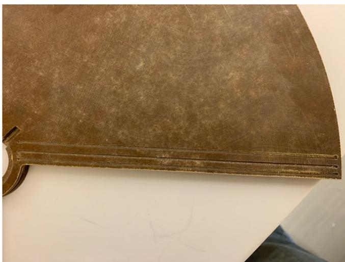
Figure 13: Slits on the rotating shutter. Three slits are placed on each side of the WGV and on both sides of the RS.
